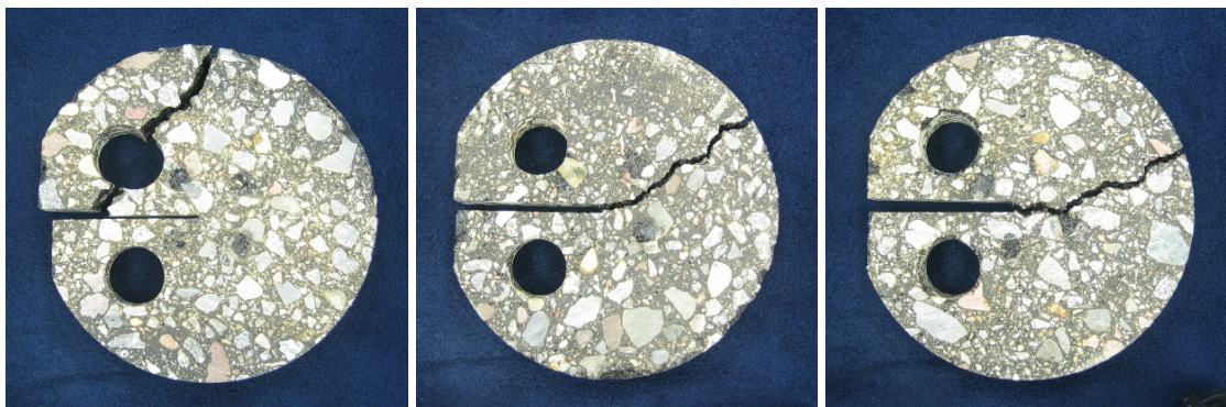
Figure 1.4. Imperfections in the Failure of DC(t) Specimens
