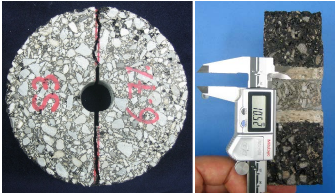
Figure 3.8. a) Fractured IRT Specimen, b) Measurement of the Initial Notch Length
